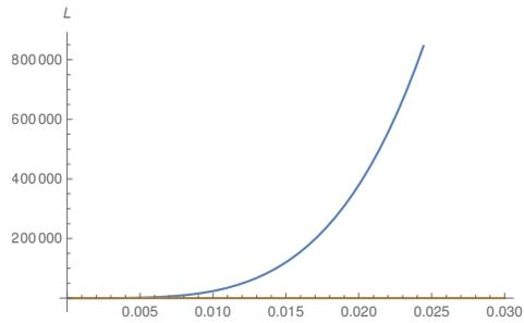
Figure 3: corrected\* Length vs radius of suspending Tungsten wire to achieve a 10 mHz resonant frequency in the original MAGPI design (moment of inertia  $I \approx 0.027 \text{ kgm}^2$ )
