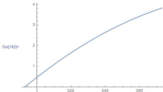
It turns out the slump in thermal conductivity of 6H SiC is insignificant compared to the possible power output gained from a larger temperature across the gradient, so the maximum distance we can place the ice bath occurs at the max permissible wire temperature of 100 deg C.
