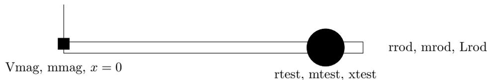
Since moment of inertia is additive, we can simply consider the moment of inertia of each component in our system about the suspension point and sum them to find the total moment. We find them by a table of moments of inertias and by the parallel axis theorem.
