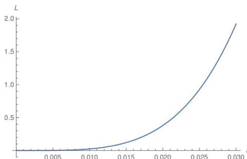
Figure 2: Length vs radius of suspending Tungsten wire to achieve a 10 mHz resonant frequency in the original MAGPI design (moment of inertia  $I \approx 0.027$  kgm<sup>2</sup>)
