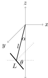
We see that the range of  $z$  spanned by the pendulum body depends on both  $\alpha$  and  $\theta$ , as thus does the total gravitational potential energy in the Lagrangian formalism.
