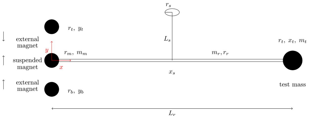
Figure 4: New MAGPI design and parameters
