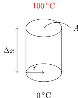
Figure 1: Depiction of a cylindrical Copper connection between the Helmholtz Loops and ice bath
