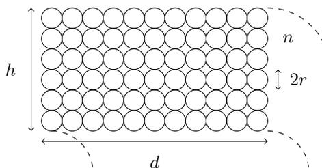
A width  $d$  can fit  $\frac{d}{2r}$  wires horizontally (we'll assume this produces an integer number), suggesting a height (dimensionless; as a number of wires)
